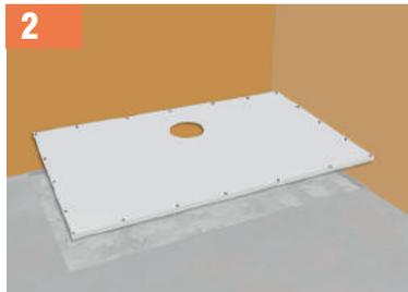
2 Excavate the floor within the marked area to a sufficient depth of **24mm** to accept ShowerDec®.
