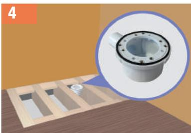
4 Connect the trap body to your outlet pipework, position between joists and centrally beneath the hole in the ShowerDec®.
