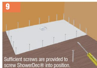
Sufficient screws are provided to screw ShowerDec® into position.
