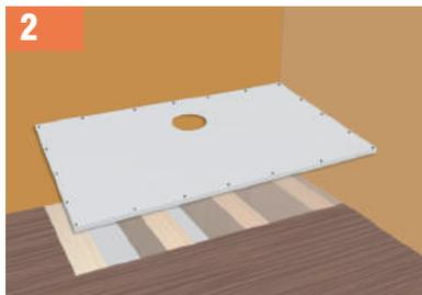
2 Remove the floor within the marked area to a depth of 18mm to accept ShowerDec®.
