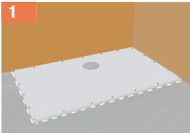
1 Locate ShowerDec® in the corner to which it is going to be finally positioned & mark lines around the outer edge.
