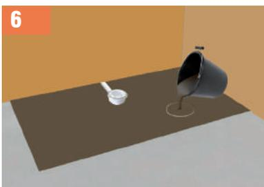
6 Apply a self levelling screed mix to cover all of the proposed area. This will ensure ShowerDec® is fully supported.
