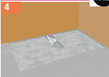
4 Remove ShowerDec®. Decide upon the position of the waste pipe knocking out a hole in the adjacent wall if required. It will be necessary to remove an area to sufficient depth under the outlet position to accommodate the shower trap. (Approximate trap depth 95mm x 110mm wide).
