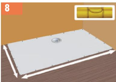
8 Ensure that the ShowerDec® is well supported and completely level.
