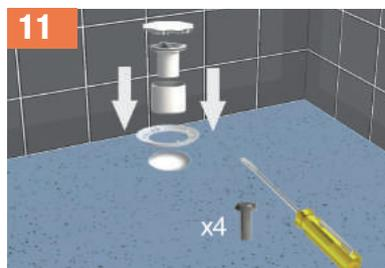
11 Once the floor covering is laid, screw into position the traps clamping ring using the bolts provided ensuring the inner cup and dip tube can still be removed.
