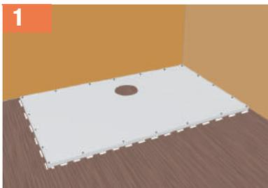
1 Locate ShowerDec® in the corner to which it is going to be finally positioned and mark lines around the outer edge.
