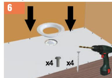
6 Attach flange to the trap body using the 4 bolts provided, ensuring that the rubber seal is in place. Secure flange to ShowerDec®, there are 4 countersunk indentations in the flange to assist with this.
