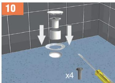
10 Once the floor covering is laid, screw into position the trap clamping ring using the bolts provided, ensuring the inner cup & dip tube can still be removed. Fit the shower traps push on cover plate.
